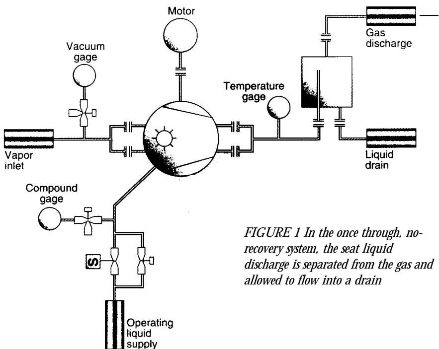
*FIGURE 1 In the once through, no-recovery system, the seal liquid discharge is separated from the gas and allowed to flow into a drain*
